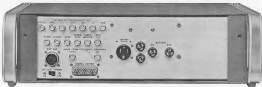
Figure 1. Type 1123-A Digital Synchronometer® time comparator, front (less bezel) and rear views.
