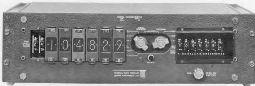
Figure 1. Type 1123-A Digital Synchronometer® time comparator, front (less bezel) and rear views.
